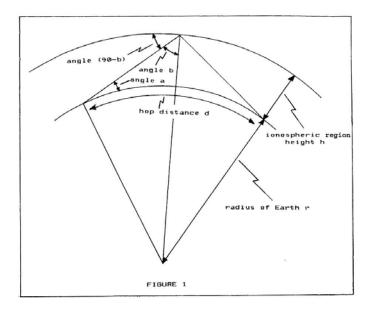
The take-off angle is the angle designated "a". The angle of incidence on the ionosphere is the angle designated "90-b". The height of the ionosphere "h" is a critical parameter in determining the M-factor. Here are some M-factors for various heights "h" at various take-off angles "a".
