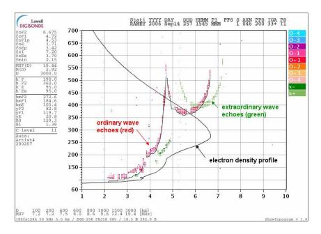
This image is from an ionosonde, which is for all intents and purposes a radar station pointing straight up. The ordinary wave swept-frequency echoes are translated into the electron density profile. For the record, this is a daytime ionogram from the Ramey (Puerto Rico) ionosonde on September 14, 2006 at 1545 UTC.
