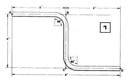
Accurate measurements coupled with exact angles must result in a tube line that will fit at points (A-D).
