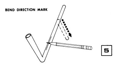
One method for keeping track of changes in plane is to use a longitudinal or lengthwise bend direction mark. (Figure 5) Put the mark on the side opposite the direction in which you wish to bend. When you put the tube in the bender, center the mark face up in the groove of the radius block. (Figure 6) This will insure that you bend in the correct direction. It also gives you a reference mark in case you must leave your work unfinished.
