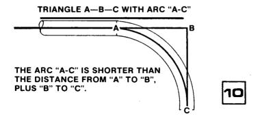
Always try to bend in the same direction -- away from the original starting end. If you reverse the direction of bending (bending towards instead of away from the original starting end) you will "trap" the stretch. Thus, if you unknowingly make a reverse bend of 90°'s, you will trap approximately one tube O.D. and increase your length between bends by that amount.
