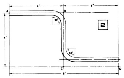
Measuring error on second leg (B-C) results in tube line that can not fit at point (D).
