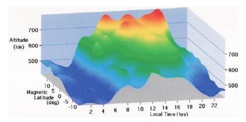
The front axis is local time. The left side axis is magnetic latitude. The vertical axis (annotated in two places) is altitude in km. The color coding denotes the magnitude of the electron density. For this set of data, the electron density minimizes around 400 km during the night, and the maximum electron density is around 800 km during the daytime.
