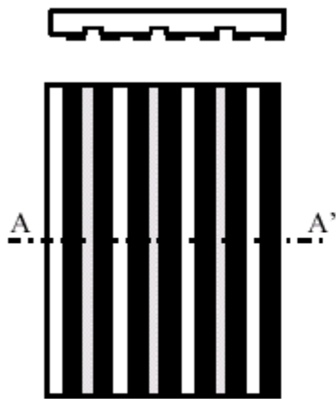
(a) Fine Pattern Mask [Levenson PSM]
