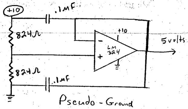
Input Filtering Stage - A/C Couples Signal and Limits Voltage Swings
