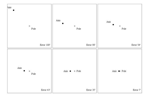
I am slowly getting better at aligning the polar axis. This last sequence required about 15 minutes to complete. Unfortunately, I haven't been able to do better than this due to poor equipment. What is needed is a better camera focus, longer exposures, longer focal length, and finer mount positioning controls (or a more delicate touch). Or perhaps just more practice.
