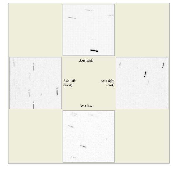
Note the apparent counter-clockwise rotation in the arrangement of photo of the drifts with respect to direction of axis misalignment. From these photos it is evident that the direction of the north pole is an angular distance in a direction about 90 degrees counter clockwise from the direction of the star trails.
